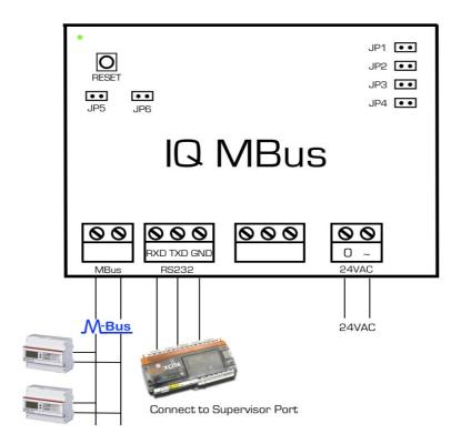
**NOTE:** The CNC supervisor port must be set to 0 on the TREND IQ controller. **NOTE:** If using a pin code: Set a user pin code to 3532 and level to 99 on the controller.
